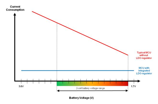
Furthermore, since power consumption is directly proportional to the switching frequency, it is important for systems designers to normalize the quoted current numbers down to a current / MHz basis. By combining these two factors, it is possible to perform a side-by-side comparison of MCUs based on the following metric:
